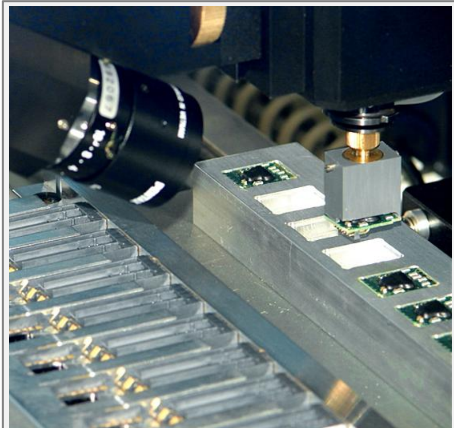
3D assembly of MID braille modules
