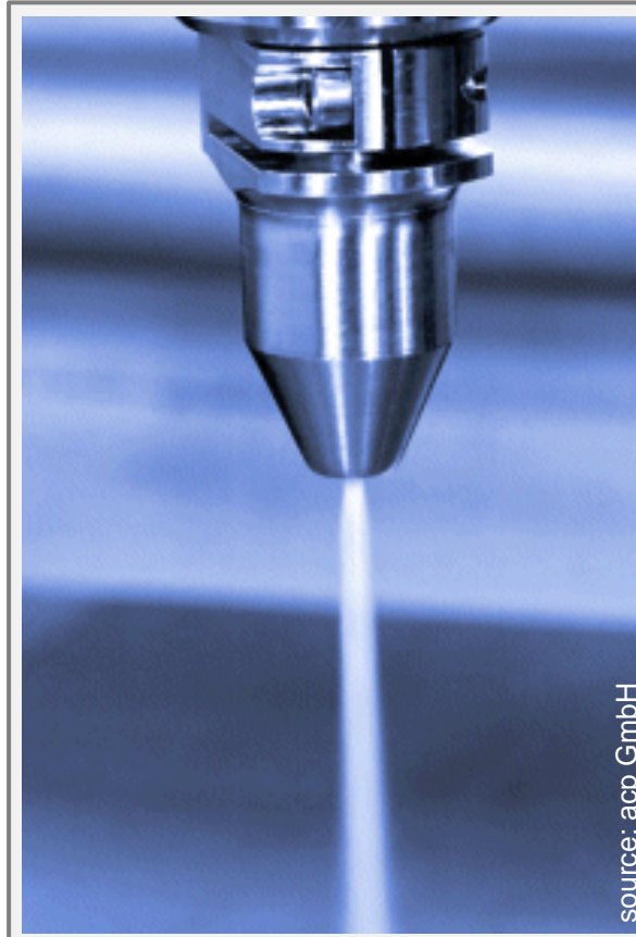
CO 2 snow jet cleaning
