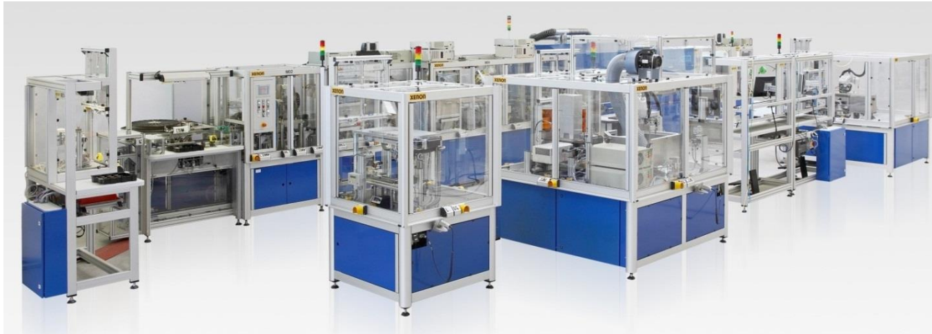
Production line for 3D-MID combi switches
